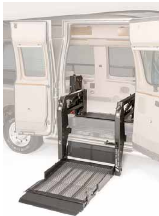
The doorway on this full-size van has been raised and equipped with a platform lift.
