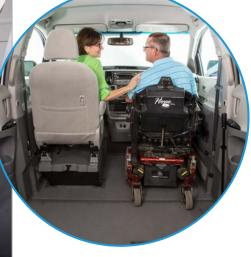
Removable front seats are equipped with rolling casters, making them easy to remove and lock back into place.
