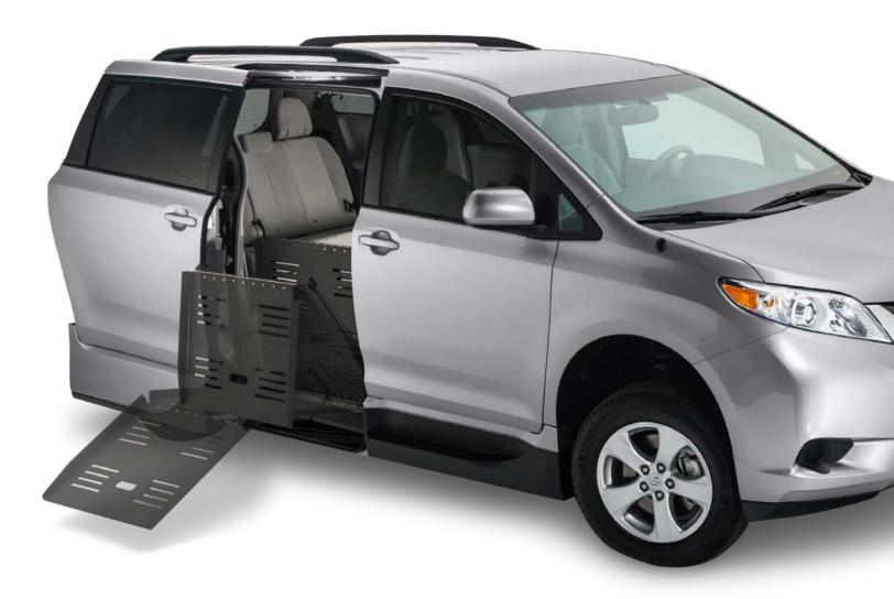
VMI also builds Toyota Sienna conversions with a traditional foldout ramp for wheelchair users who prefer taller ramp side rails. The Summit is more reliable than ever before with a stronger, more robust fold-out ramp and stainless steel hardware that resists corrosion. The Summit conversion offers superior usability to that of any other Toyota Sienna fold-out ramp conversion.
