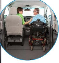
Removable front seats are equipped with rolling casters, making them easy to remove and lock back into place.
