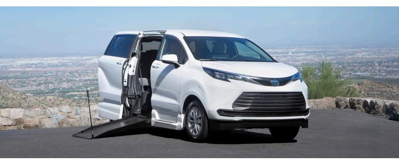
The economical Northstar E manual in-floor ramp is easy to deploy and stow, while offering generous space for wheelchair maneuverability inside the cabin. Plus, enjoy added flexibility with a removable front passenger seat and core Toyota Sienna features like Toyota Safety Sense 2.0, an 8" touchscreen, and more.
